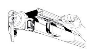
13) Slide steel installation plates to the groove in front bar and secure both ends with front bar end caps (PVC). Secure end caps with M3.5x16 screws.
