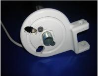
If it is necessary to change drive sides (pin is in the bracket on which you want to install the drive) the pin should be put into the opposite bracket (change bracket axis with pin installation (b) for bracket axis (a). Both parts will be changed by undoing (de-installation) and securing (installation) of M22 nut with washer.
