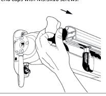
14) With spirit level check if the arms close to one plane on a slightly opened awning. If necessary adjust the arm level by loosening or tightening the internal M5 screw in universal brackets.
