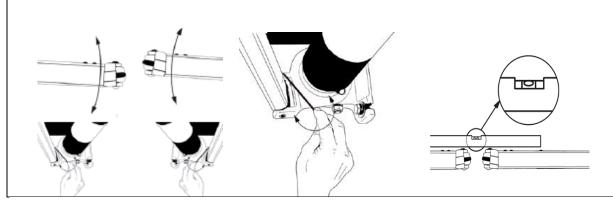
15) To change awning tilt angle open it completely, then loosen M22 nuts in brackets. With flat wrench loosen (to increase tilt angle) or tighten (to decrease tilt angle) regulation screws in brackets.
